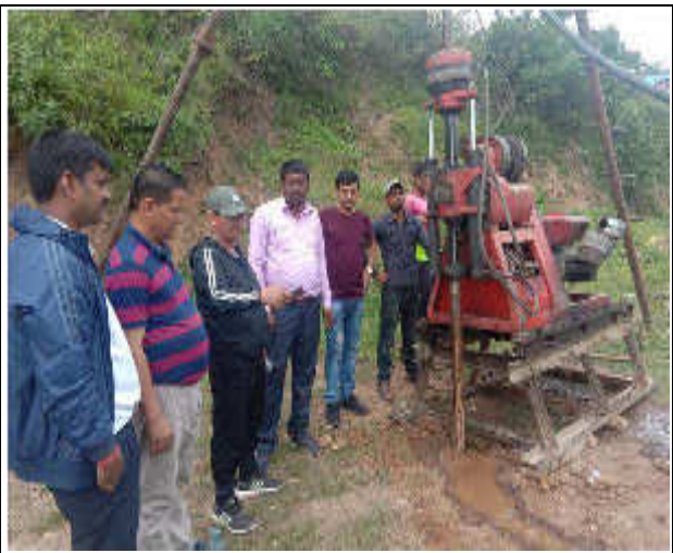
Photo 2: Geotechnical investigation and SPT test of soil by borehole drilling at Ilam
